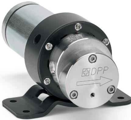
The Optima series is designed for applications requiring a very small package size. The construction is the same as those of its larger cousins, but by removing one of the shaft bearings the overall length is much shorter. The inlet and outlet ports can be located on the side or end of the pump, and are available in a variety of sizes. The brushstyle DC motor is oversized and gives excellent brush life at optimum price-performance-ratio.
