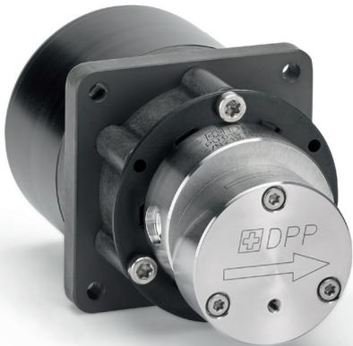
The Optima series is designed for applications requiring a very small package size. The construction is the same as those of its larger cousins, but by removing one of the shaft bearings the overall length is much shorter. The inlet and outlet ports can be located on the side or end of the pump, and are available in a variety of sizes. The brush-less DC motor has an integral flange allowing bulkhead mounting, and its IP-55 rating ensures it will stand up to harsh environments.
